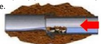
Misaligned - Offset Pipe Joint
